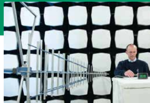
Our semi-anechoic chamber complies with the latest EMC and radio standards
