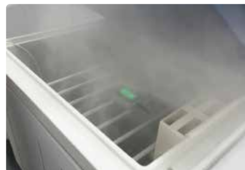
Salt mist testing - especially used for marine equipment
